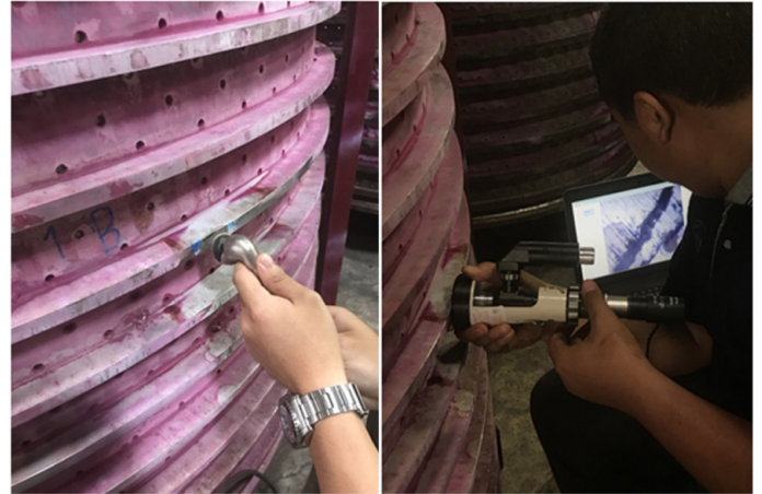
Figure3:Grinding process in MicrostructureAnalysis technique Figure4:Using portable microscope to analyse micrograph
