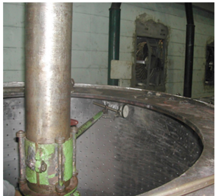
1 Permanent magnet motor | 2 Feeding pipe used for massecurite orientation 3 Casing | 4 Basket | 5 Booster Distribution.
